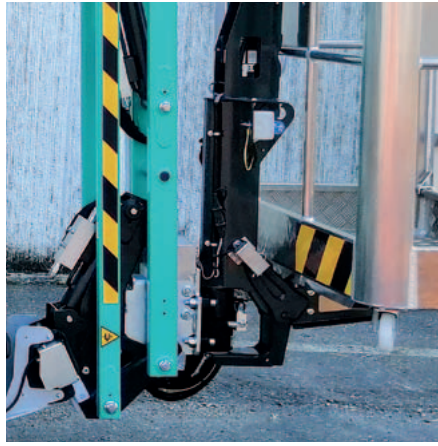
Compactness of the jib assembly hosting both the load cell and basket rotation system.
