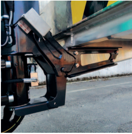
Basket mounting system designed for easiness of assembly.
